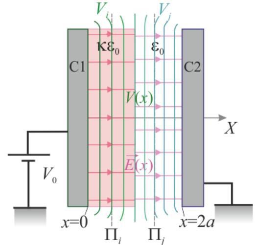
$$P(x_i, y, z) \in \Pi_i : x = x_i, \text{ tal que } d\vec{r}|_{\Pi_i} = dy\vec{j} + dz\vec{k} \perp \vec{E}(P) \parallel \vec{i} \implies \left\{ \begin{array}{l} dV|_{\Pi_i} = -\vec{E}(P) \cdot d\vec{r}|_{\Pi_i} = 0 \\ V(x, y, z)|_{\Pi_i} = V(x = x_i) = V_i, \text{ cte.} \end{array} \right.$$
