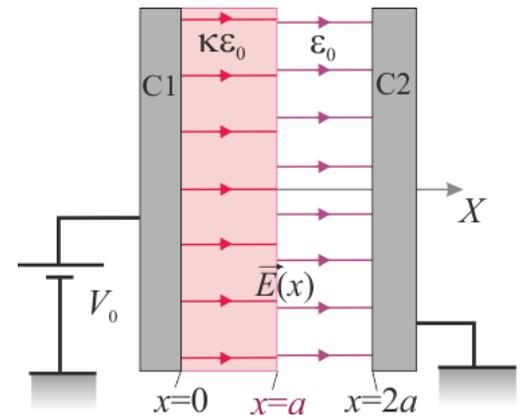
$$\vec{E}(x, y, z) = \begin{cases} \frac{E_0}{\kappa} \vec{i}; & \text{si } 0 < x < a \\ E_0 \vec{i}; & \text{si } a < x < 2a \end{cases}$$
